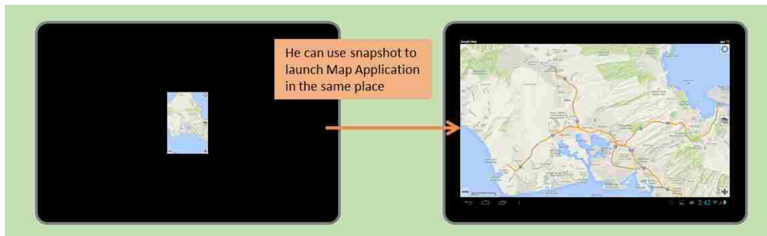
Figure 6 - If a user has the same application on his own device, he can use the snapshot to launch the application to that state.
